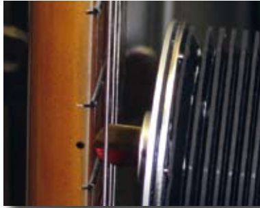
Sensorfinger: With the Plek scan the machine makes a „digital fingerprint“ of the fretboard.
